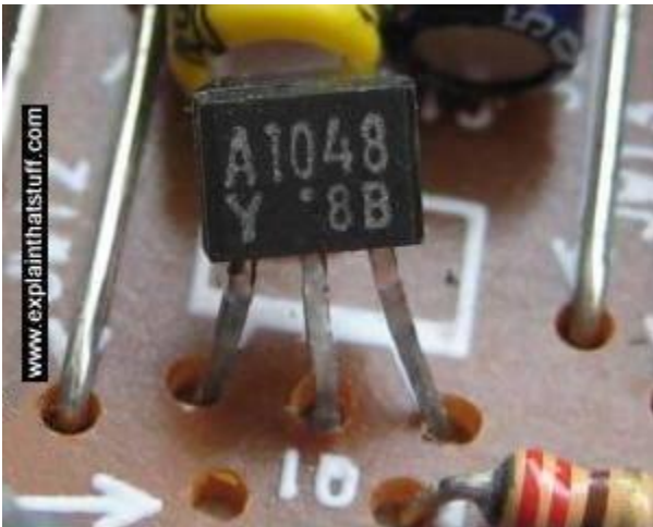
Photo: A typical transistor on an electronic circuit board.
